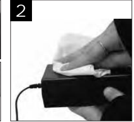
2 Wipe AC to DC adapter housing and cords with a dry cloth.
